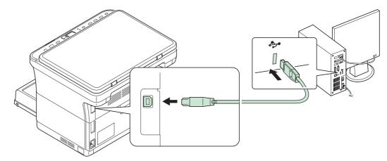
**Note** Use a USB cable with a rectangular Type A plug and a square Type B plug. The USB cable should be shielded and no longer than 5 meters (16 feet) long.
